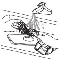
3. Larger food remnants can be cleaned by rinsing the filter under running water.
